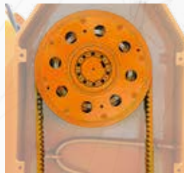
Centrifugal clutch suggested with forestry rotor
