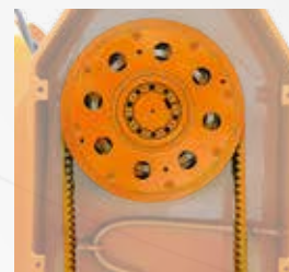
Centrifugal clutch recommended with forestry rotor
