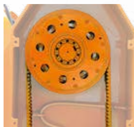
Centrifugal clutch recommended with forestry rotor
