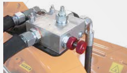
Hydraulic transmission of pick-up rotor and speed regulator
