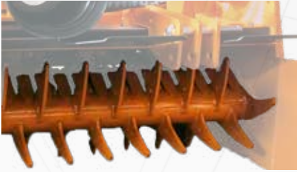
Pick-up rotor with extra-quantity of teeth
