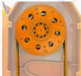
Centrifugal clutch suggested with forestry rotor
