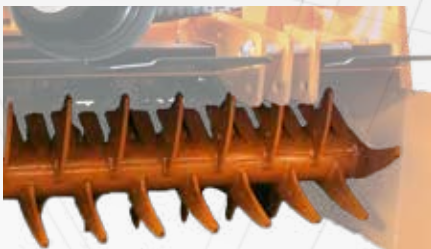
Pick-up rotor with extra-quantity of teeth
