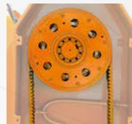
Centrifugal clutch recommended with forestry rotor
