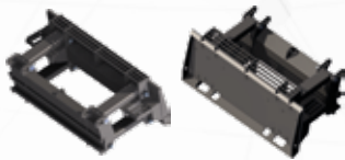
Self-levelling skid steer mount with parallel arms (SAE J2513)
